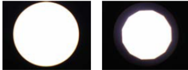
Figure 9: These images compare what the image will look at before opening the aperture diaphragm (left) and after closing the aperture diaphragm to 80% (right).
